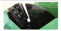
**Easy access** to blades and clearing of housing, a few turns of the wingnut and everything is accessible within seconds.
